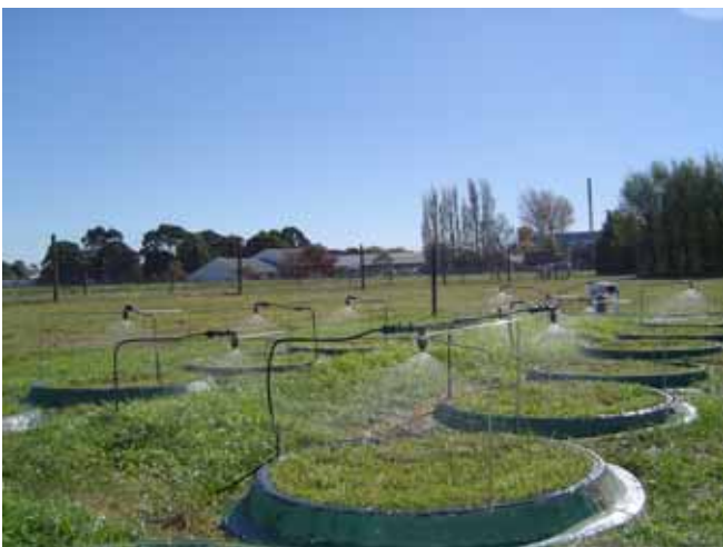
Figure 1. Irrigation being applied to eight of the 16 lysimeters.
