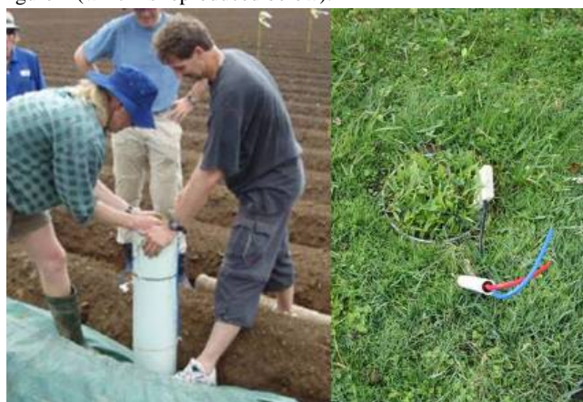
Figure 4. The use of water flux meters in the field. Left: Installation of a water flux meter under potatoes. Right: A water flux meter under pasture. The protruding tubes are for the calibration of the tipping spoon (light-coloured tube) and the extraction of the soil solution (darker tube). Additionally, a CS616 soil moisture sensor (see Chapter 16) was installed to measure the soil's water content.
